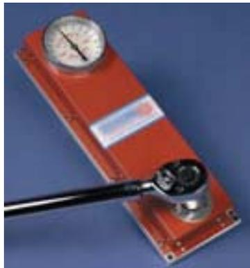
**Cary Code# 30B5TT** - 0 to 50 Ft/Lb. Torque Wrench Tester - **Model#: TAF-50**
