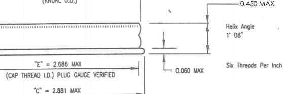
The Max & Min. inside diameter of the thread are determined by round Max & Min plug gauges. The closure should permit entry of the min gauge and no entry with a slight drag on the max gauge.
