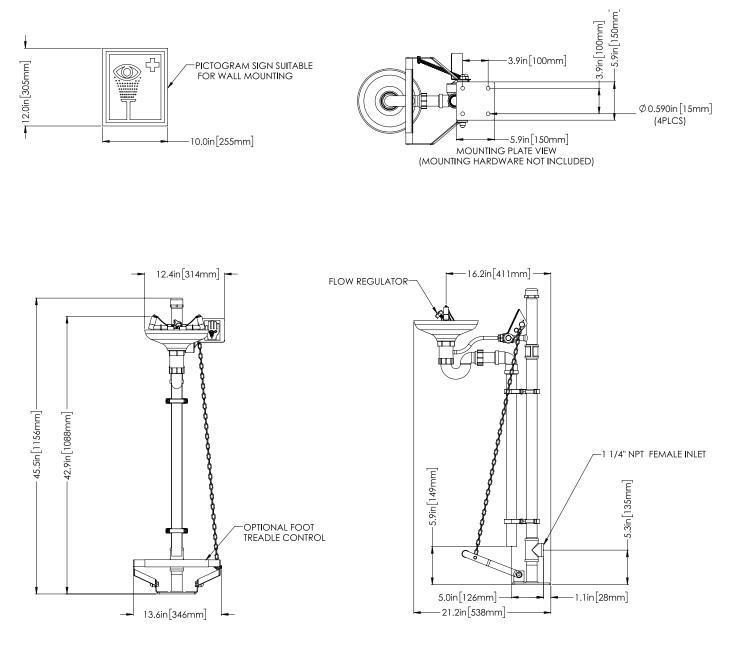
VARIATIONS IN MANUFACTURING AND ASSEMBLY ALLOW FOR  $\pm 1/8$  IN [3MM] PER THREADED JOINT.
