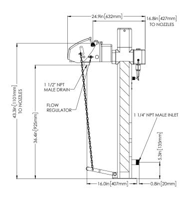
VARIATIONS IN MANUFACTURING AND ASSEMBLY ALLOW FOR ±1/8 in [3 mm] PER THREADED JOINT.
