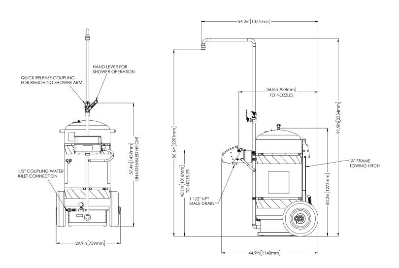
VARIATIONS IN MANUFACTURING AND ASSEMBLY ALLOW FOR  $\pm 1/8$  in [3 mm] PER THREADED JOINT.
