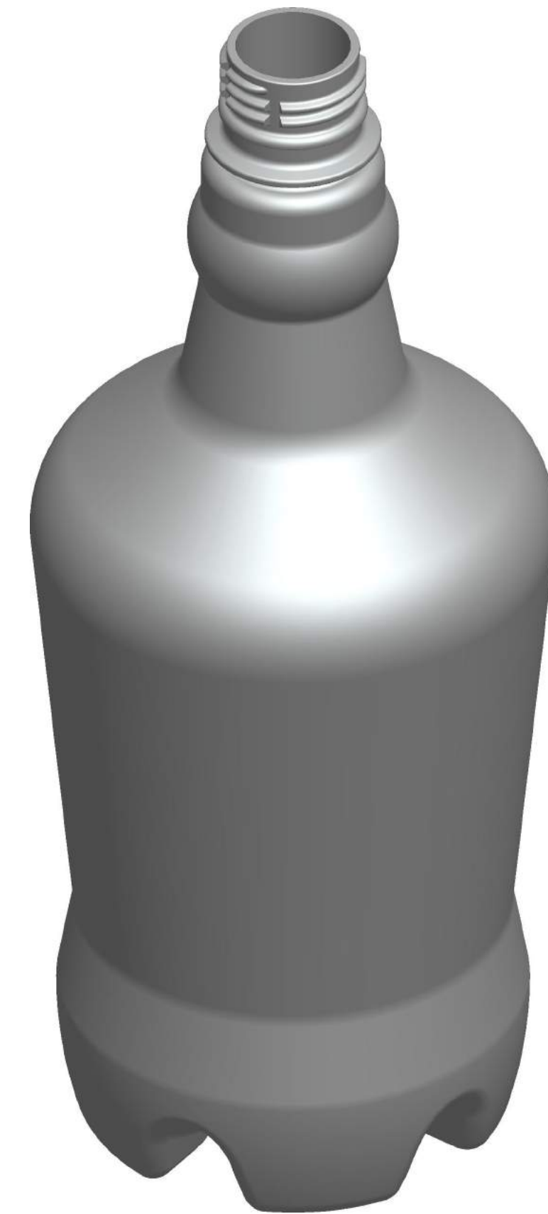
DETAIL A PCO-1810 NECK FINISH 2-1/4 THREAD TURNS X 8 T.P.I. SCALE 2.000
