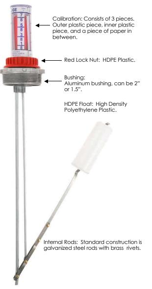
Top mounted liquid level gauge that can measure from 6 inches to 144 inches in depth. Bushing size can be 2" or 1.5". Gauges are custom made in house to fit your tank. Can also accommodate for double walls and pipe risers. <u>The</u> <u>Type H Gauge has a 2 piece bushing construction that</u> <u>allows you to aim your swing arm away from walls, corners,</u> <u>and other obstructions.</u>
