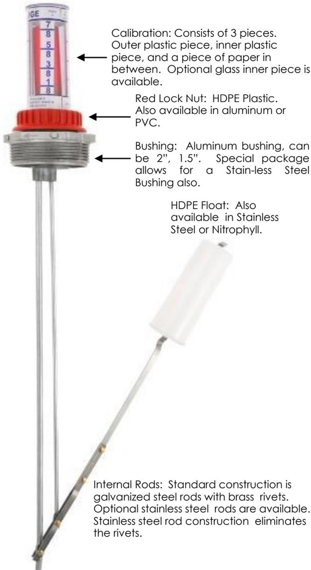
Calibration: Consists of 3 pieces. Outer plastic piece, inner plastic piece, and a piece of paper in between. Optional glass inner piece is available.
